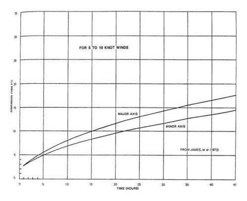
Figure 7-1. Growth of a 500 ton oil spill during five to ten knot winds.
