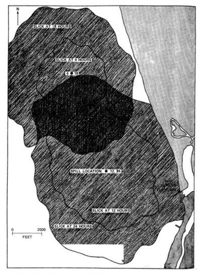
Figure 7-5. Predicted behavior of a 500 ton oil spill under calm winds and a 0.3 knot tidal current (spill initiated at slack water before flood tide).
